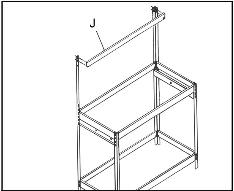
8. Assemble the remaining top long beam (J) to the left/right top side beams (K/L).
